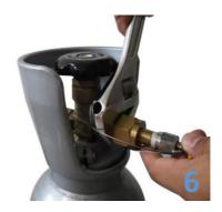
Put a rubber sealing ring in the nut of the dry ice maker and then connect the nut to the CO2 cylinder, use your fingers to screw tight until you can't screw.
