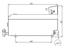
Power Connection **Net Weight** 27 kg Machine Dimensions W600 x D600 x H380 mm HS Customs Code EAN Code **Article Number**
